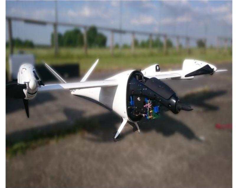
MACS Camera system module mounted In front of the fixed-wings drone
